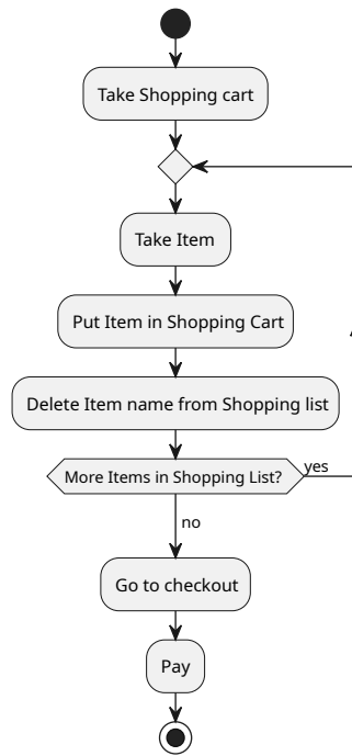
Figure 68: Example of an activity diagram
